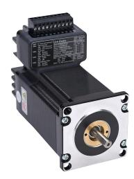
SureStep DC integrated stepper motor/drive, microstepping, NEMA 23 frame, IP20, 5A, 12-48 VDC, bipolar, 210 oz-in holding torque, 1.8-degree step angle, 200 to 25000 steps per revolution.
