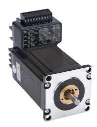
SureStep DC integrated stepper motor/drive, microstepping, NEMA 23 frame, IP20, 5A, 12-48 VDC, bipolar, 210 oz-in holding torque, 1.8-degree step angle, 200 to 25000 steps per revolution, external (field-wireable) encoder.
