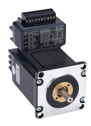
SureStep DC integrated stepper motor/drive, microstepping, NEMA 23 frame, IP20, 5A, 12-48 VDC, bipolar, 125 oz-in holding torque, 1.8-degree step angle, 200 to 25000 steps per revolution.
