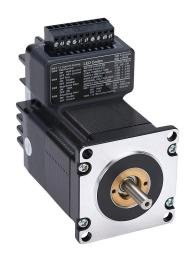
SureStep DC integrated stepper motor/drive, microstepping, NEMA 23 frame, IP20, 5A, 12-48 VDC, bipolar, 125 oz-in holding torque, 1.8-degree step angle, 200 to 25000 steps per revolution, external (field-wireable) encoder.
