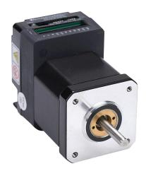
SureStep DC integrated stepper motor/drive, microstepping, NEMA 17 frame, IP20, 2A, 12-48 VDC, bipolar, 68 oz-in holding torque, 1.8-degree step angle, 200 to 25000 steps per revolution.
