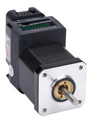
SureStep DC integrated stepper motor/drive, microstepping, NEMA 17 frame, IP20, 2A, 12-48 VDC, bipolar, 68 oz-in holding torque, 1.8-degree step angle, 200 to 25000 steps per revolution, external (field-wireable) encoder.
