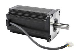
SureStep stepper motor, NEMA 42 frame, IP40, single shaft, 8A, 4532 oz-in holding torque, 1.8-degree step angle, 200 steps per revolution, bipolar. Requires SureStep STP-EXT42H-xxx cable.
