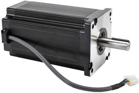
SureStep stepper motor, NEMA 42 frame, IP40, single shaft, 8A, 4532 oz-in holding torque, 1.8-degree step angle, 200 steps per revolution, bipolar. Requires SureStep STP-EXT42H-xxx cable.
