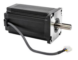
SureStep stepper motor, NEMA 42 frame, IP40, dual shaft, encoder ready, 8A, 4532 oz-in holding torque, 1.8-degree step angle, 200 steps per revolution, bipolar. Requires SureStep STP-EXT42H-xxx cable.
