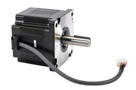
SureStep stepper motor, NEMA 42 frame, IP40, single shaft, 6A, 1742 oz-in holding torque, 1.8-degree step angle, 200 steps per revolution, bipolar. Requires SureStep STP-EXT42H-xxx cable.
