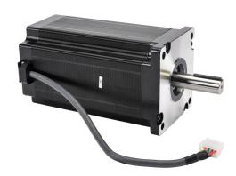
SureStep stepper motor, NEMA 42 frame, IP40, single shaft, 6A, 4390 oz-in holding torque, 1.8-degree step angle, 200 steps per revolution, bipolar. Requires SureStep STP-EXT42-xxx cable.
