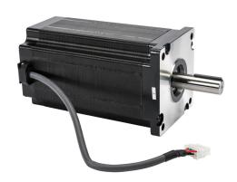
SureStep stepper motor, NEMA 42 frame, IP40, dual shaft, encoder ready, 6A, 4390 oz-in holding torque, 1.8-degree step angle, 200 steps per revolution, bipolar. Requires SureStep STP-EXT42-xxx cable.
