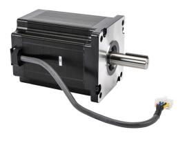
SureStep stepper motor, NEMA 42 frame, IP40, single shaft, 6A, 3116 oz-in holding torque, 1.8-degree step angle, 200 steps per revolution, bipolar. Requires SureStep STP-EXT42-xxx cable.
