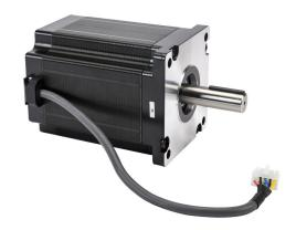
SureStep stepper motor, NEMA 42 frame, IP40, dual shaft, encoder ready, 6A, 3116 oz-in holding torque, 1.8-degree step angle, 200 steps per revolution, bipolar. Requires SureStep STP-EXT42-xxx cable.
