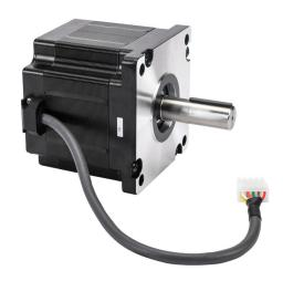
SureStep stepper motor, NEMA 42 frame, IP40, single shaft, 4.2A, 1728 oz-in holding torque, 1.8-degree step angle, 200 steps per revolution, bipolar. Requires SureStep STP-EXT42-xxx cable.
