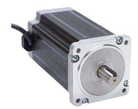
SureStep stepper motor, NEMA 34 frame, IP40, single shaft, 2.5A, 1841 oz-in holding torque, 1.8-degree step angle, 200 steps per revolution, bipolar.
