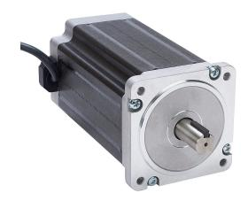
SureStep stepper motor, NEMA 34 frame, IP40, single shaft, 2.5A, 1841 oz-in holding torque, 1.8-degree step angle, 200 steps per revolution, bipolar.
