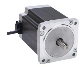
SureStep stepper motor, NEMA 34 frame, IP40, single shaft, 2.05A, 1110 oz-in holding torque, 1.8-degree step angle, 200 steps per revolution, bipolar.
