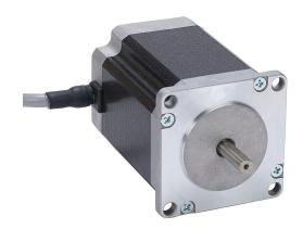
SureStep stepper motor, NEMA 23 frame, IP40, single shaft, 0.71A, 227 oz-in holding torque, 1.8-degree step angle, 200 steps per revolution, bipolar.
