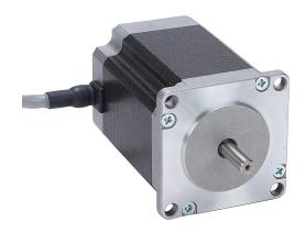
SureStep stepper motor, NEMA 23 frame, IP40, dual shaft, encoder ready, 0.71A, 227 oz-in holding torque, 1.8-degree step angle, 200 steps per revolution, bipolar.
