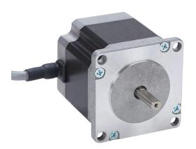
SureStep stepper motor, NEMA 23 frame, IP40, single shaft, 0.71A, 149 oz-in holding torque, 1.8-degree step angle, 200 steps per revolution, bipolar.
