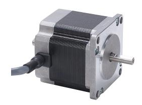
SureStep stepper motor, NEMA 23 frame, IP40, dual shaft, encoder ready, 0.71A, 149 oz-in holding torque, 1.8-degree step angle, 200 steps per revolution, bipolar.
