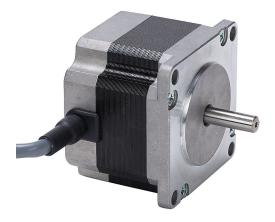
SureStep stepper motor, NEMA 23 frame, IP40, single shaft, 0.71A, 75 oz-in holding torque, 1.8-degree step angle, 200 steps per revolution, bipolar.
