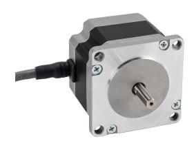
SureStep stepper motor, NEMA 23 frame, IP40, dual shaft, encoder ready, 0.71A, 75 oz-in holding torque, 1.8-degree step angle, 200 steps per revolution, bipolar.
