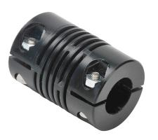
AutomationDirect encoder/stepper coupling, 3/8in to 1/2in bore, engineered polymer body, setscrew. For use with Koyo TRDA-20 and TRDA-25 series encoders and NEMA size 34 stepper motors.
