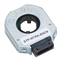
SureStep incremental (quadrature) rotary modular encoder, 5 VDC, radial exit, line driver (differential) output, up to 4096 ppr, software configurable. For use with NEMA 14, 17, and 23 SureStep dual shaft motors.
