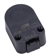
SureStep incremental (quadrature) rotary modular kit encoder, 5 VDC, radial exit, push-pull (totem) output, 400 ppr. For use with SureStep stepper motors with 1/4in rear shaft.
