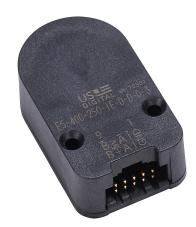
SureStep incremental (quadrature) rotary modular kit encoder, 5 VDC, radial exit, line driver (differential) output, 400 ppr. For use with SureStep stepper motors with 1/4in rear shaft.
