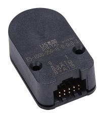
SureStep incremental (quadrature) rotary modular kit encoder, 5 VDC, radial exit, line driver (differential) output, 1000 ppr. For use with SureStep stepper motors with 1/4in rear shaft.
