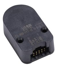
SureStep incremental (quadrature) rotary modular kit encoder, 5 VDC, radial exit, line driver (differential) output, 400 ppr. For use with SureStep stepper motors with 5mm rear shaft.
