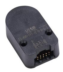
SureStep incremental (quadrature) rotary modular kit encoder, 5 VDC, radial exit, line driver (differential) output, 400 ppr. For use with SureStep stepper motors with 5mm rear shaft.
