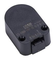
SureStep incremental (quadrature) rotary modular kit encoder, 5 VDC, radial exit, push-pull (totem) output, 1000 ppr. For use with SureStep stepper motors with 5mm rear shaft.
