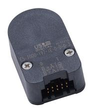
SureStep incremental (quadrature) rotary modular kit encoder, replacement, 5 VDC, radial exit, line driver (differential) output, 1000 ppr. For use with SureStep stepper motors with 5mm rear shaft.
