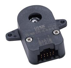
SureStep incremental (quadrature) rotary modular kit encoder, 5 VDC, radial exit, line driver (differential) output, 400 ppr. For use with SureStep stepper motors with 3/8in rear shaft.
