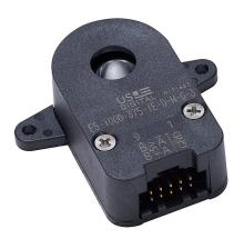
SureStep incremental (quadrature) rotary modular kit encoder, 5 VDC, radial exit, line driver (differential) output, 1000 ppr. For use with SureStep stepper motors with 3/8in rear shaft.
