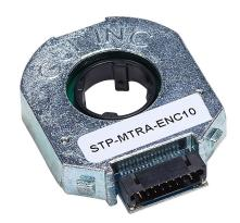
SureStep incremental (quadrature) rotary modular encoder, 5 VDC, radial exit, push-pull (totem) output, up to 4096 ppr, software configurable. For use with NEMA 14, 17, and 23 SureStep dual shaft motors.
