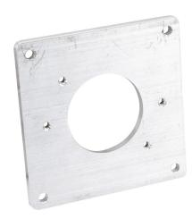
SureStep encoder mounting plate, metal body. For use with SureStep NEMA 42 stepper motors with dual shafts. Encoder mounting screws and mounting plate screws included. Mounting holes for CUI Devices AMT132/AMT332 encoders and US Digital E6 encoders.
