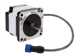
SureStep stepper motor, NEMA 34 frame, IP65, single shaft, 2.8A, 434 oz-in holding torque, 1.8-degree step angle, 200 steps per revolution, bipolar. Requires STP-EXTW-xxx cable.
