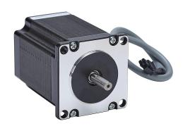
SureStep stepper motor, NEMA 23 frame, IP40, single shaft, 2.8A, 276 oz-in holding torque, 1.8-degree step angle, 200 steps per revolution, bipolar. Requires STP-EXT-xxx cable.
