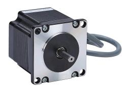
SureStep stepper motor, NEMA 23 frame, IP40, single shaft, 2.8A, 166 oz-in holding torque, 1.8-degree step angle, 200 steps per revolution, bipolar. Requires STP-EXT-xxx cable.
