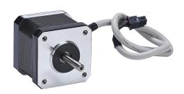
SureStep stepper motor, NEMA 17 frame, IP40, single shaft, 1.7A, 61 oz-in holding torque, 1.8-degree step angle, 200 steps per revolution, bipolar. Requires STP-EXT-xxx cable.
