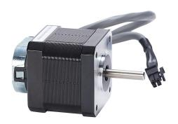
SureStep stepper motor, NEMA 17 frame, IP40, dual shaft, external (field-wireable) encoder, 1.7A, 61 oz-in holding torque, 1.8-degree step angle, 200 steps per revolution, bipolar. Requires STP-EXT-xxx and STP-CBL-EBxxx cables.
