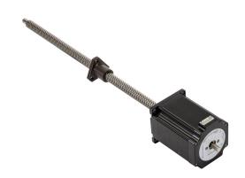
SureStep stepper motor linear actuator, external nut, encoder ready, NEMA 23 frame, IP40, triple stack, 3A, 12in lead screw length, 1in/rev, 0.5in lead screw diameter, screw code K, journal and groove end machining.
