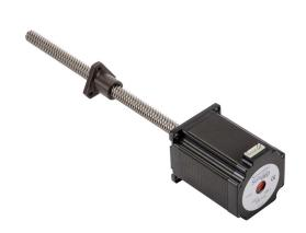
SureStep stepper motor linear actuator, external nut, NEMA 23 frame, IP40, triple stack, 3A, 9in lead screw length, 1in/rev, 0.5in lead screw diameter, screw code K, no end machining.
