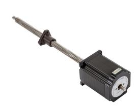
SureStep stepper motor linear actuator, external nut, encoder ready, NEMA 23 frame, IP40, triple stack, 3A, 9in lead screw length, 1in/rev, 0.5in lead screw diameter, screw code K, journal and groove end machining.
