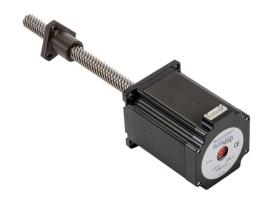
SureStep stepper motor linear actuator, external nut, NEMA 23 frame, IP40, triple stack, 3A, 6in lead screw length, 1in/rev, 0.5in lead screw diameter, screw code K, no end machining.
