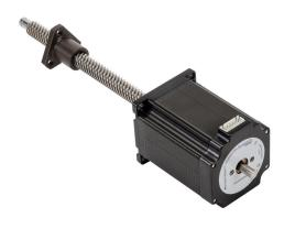
SureStep stepper motor linear actuator, external nut, encoder ready, NEMA 23 frame, IP40, triple stack, 3A, 6in lead screw length, 1in/rev, 0.5in lead screw diameter, screw code K, journal and groove end machining.
