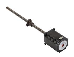
SureStep stepper motor linear actuator, external nut, NEMA 23 frame, IP40, triple stack, 3A, 12in lead screw length, 6mm/rev, 12mm lead screw diameter, screw code H, no end machining.
