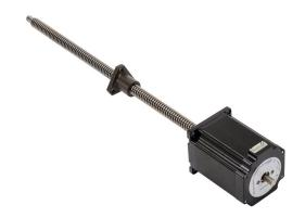
SureStep stepper motor linear actuator, external nut, encoder ready, NEMA 23 frame, IP40, triple stack, 3A, 12in lead screw length, 6mm/rev, 12mm lead screw diameter, screw code H, journal and groove end machining.
