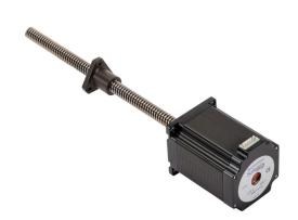
SureStep stepper motor linear actuator, external nut, NEMA 23 frame, IP40, triple stack, 3A, 9in lead screw length, 6mm/rev, 12mm lead screw diameter, screw code H, no end machining.
