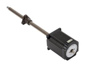
SureStep stepper motor linear actuator, external nut, encoder ready, NEMA 23 frame, IP40, triple stack, 3A, 9in lead screw length, 6mm/rev, 12mm lead screw diameter, screw code H, journal and groove end machining.
