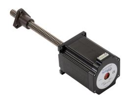
SureStep stepper motor linear actuator, external nut, NEMA 23 frame, IP40, triple stack, 3A, 6in lead screw length, 6mm/rev, 12mm lead screw diameter, screw code H, no end machining.
