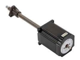
SureStep stepper motor linear actuator, external nut, encoder ready, NEMA 23 frame, IP40, triple stack, 3A, 6in lead screw length, 6mm/rev, 12mm lead screw diameter, screw code H, journal and groove end machining.
